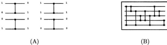
Fig. 1. (A) A 2x1 (2 inputs with 1 gate) sorting network with all possible inputs and outputs. Values propagate along the horizontal lines until they encounter a gate (vertical line), at that point the gate may switch the values or pass them through. All 1's are sorted to the bottom and all zeros to the top. A valid sorting network will correctly sort all possible inputs. (B) A 5x9 (5 inputs with 9 gates) sorting network demonstrating a larger arrangement of compare exchange gates and inputs.
